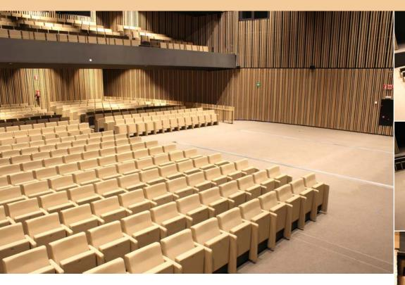
Check the custom design chair created by ASCÉNDER for this venue: chairs are mounted on an aluminium beam that moves along the rails previously installed into the floor. So, the venue can be totally emptied in minutes while concealing the chairs under the stage. Additionally, all chairs have a large foldable writing desk concealed in the back - so the venue gets the possibility of being used also as a conference venue.
